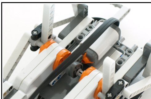
Figure 5: A Touch Sensor for leg synchronization
